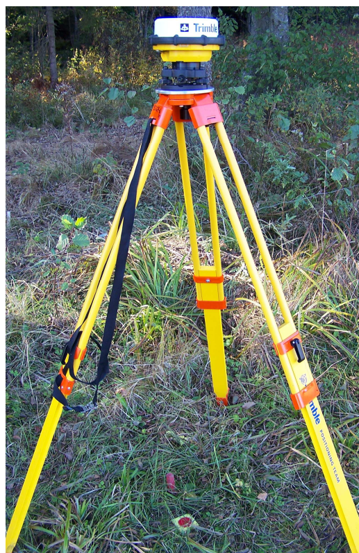
Obr. 12 GPS stanice Trimble 4600LS
