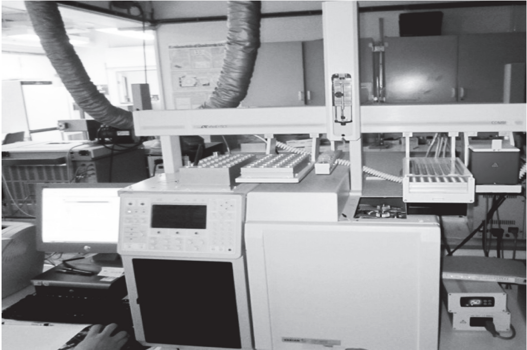
Figure 9. Gas chromatograph Varian CP 3800 used for analysing the fatty acid composition.
