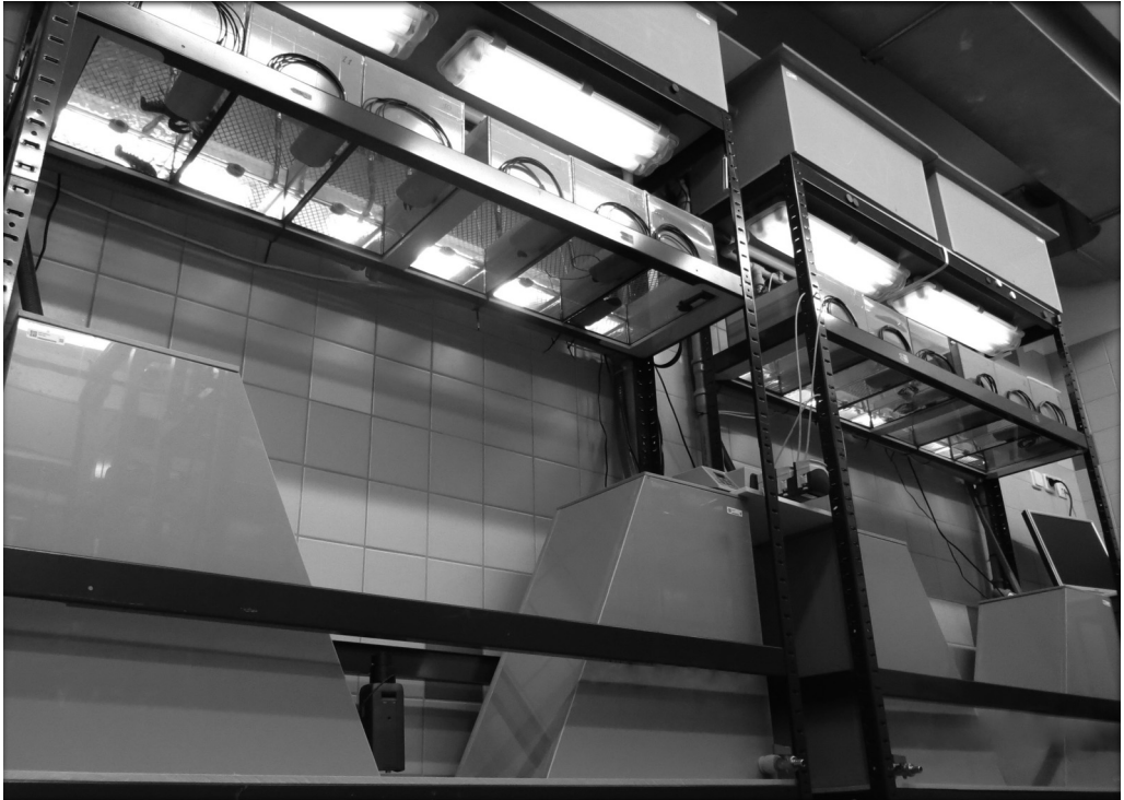
Figure 3. Experimental biomonitoring system for noninvasive recording and analysis of crayfish cardiac and behavioural activities.
