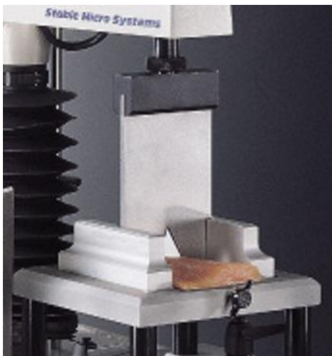
Obr. 3. Warner-Bratzlerův shear test (Stable micro systems at the forefront of fish texture testing, 2011).
