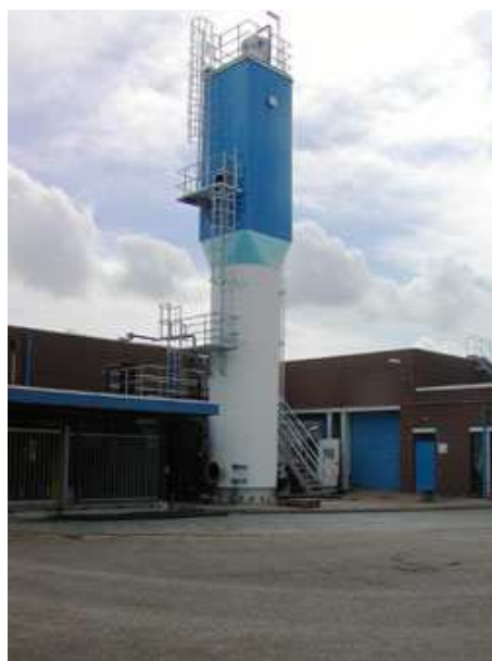
Obr. 4 : Anammox reaktor (1800 m 3 ) v Rotrdamu ( www.anammox.com/application.html ).
