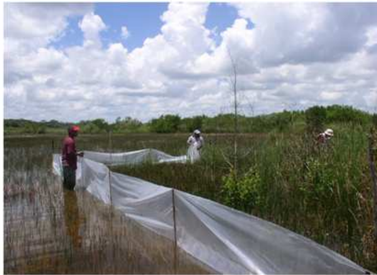
Fig. 5 P addition procedure, here in Typha plot (August 2005). Plastic barrier was installed for the period of 14 days to prevent P outflow from the defined plot.
