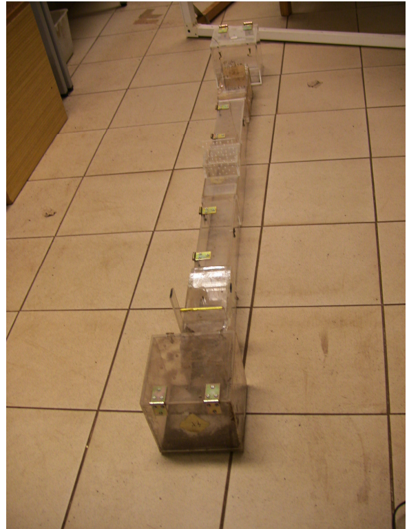
Figure 3.: Perspex tunnel, in the middle divided by perforated partition
