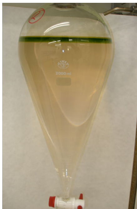
Figure 3.5. Completed partitioning of 50% MeOH extract in ratio 2:1:3 (extract: EtOAc:water) right before collecting the lower (pink) phase.
