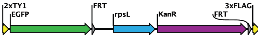
Fig. 1: Structure of the tagging cassette used for recombineering of FlyFos clones. The cassette allows recombination of EGFP either or N-terminal or C-terminal. The amplified region contains 2xTY1 and 3xFLAG sequences as internal tag for immunoprecipitation, EGFP sequence without stop codon. Kanamycin resistance and rpsL flanked with FRT for flip-out of the selection markers. Modified from Ejsmont et al., 2009.
