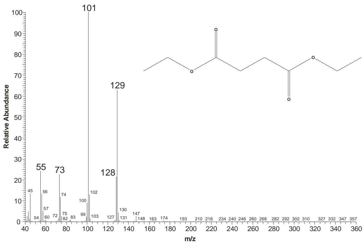
Fig. 11: GC-MS analysis, ECF derivatization, EI spectrum – succinic acid
