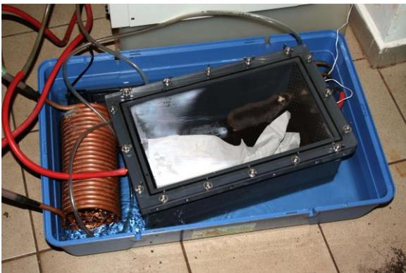
Fig. 1S. Metabolic chamber (11.8 l) submerged in the water bath.
