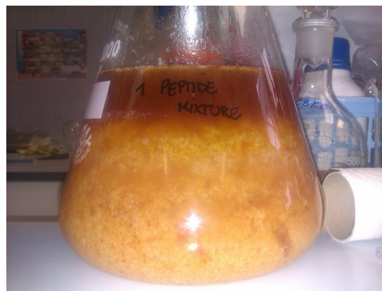
Figure 6.2: The mycelium fungal material of the Isaria strain PFR-97 after extraction and before filtration of the BVDs.
