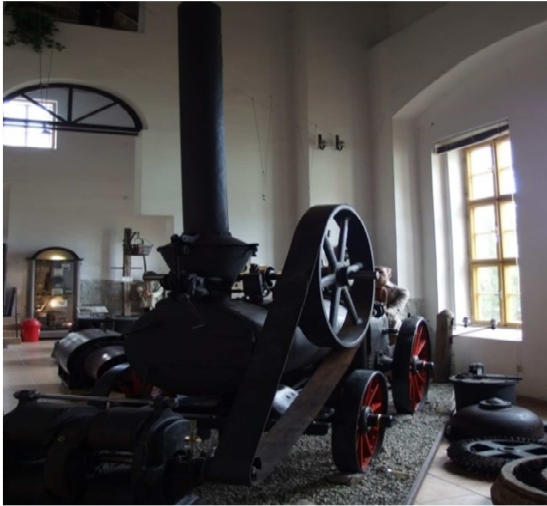
Obr. 4.4.3 Lokomobila s dynamem
