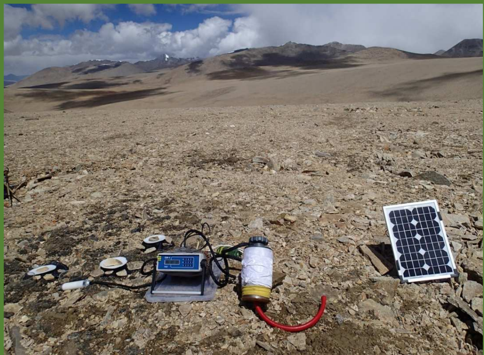
Field measuring of the metabolic activity of BSCs in dark/light conditions using the EGM4 Gas Analyser (Tibetan plateau, 5900m a.s.l.).
