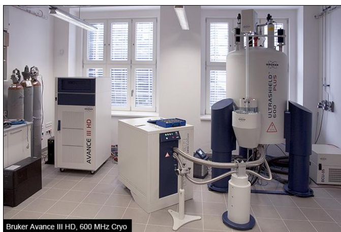
Figure 14. An image of the Bruker Avance III HD, 600 MHz spectrometer (image courtesy of www.uochb.cz ).
