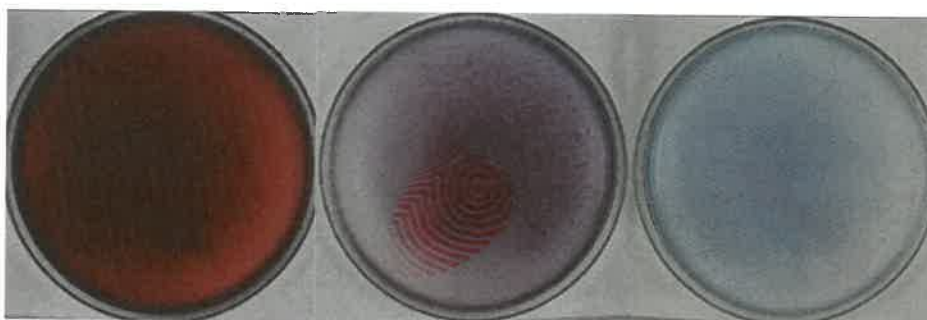
Fig. 1. The system starts out in a reducing state (left, indicated by and red color of ferroin) and reaches equilibrium in an oxidized state (right, blue color by ferriin)
