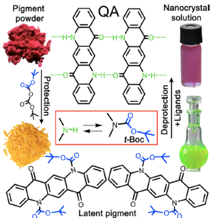
Figure 8: The synthetic route to produce colloidal solutions from pigment crystals on the example of quinacridone. (Taken from 32 )
