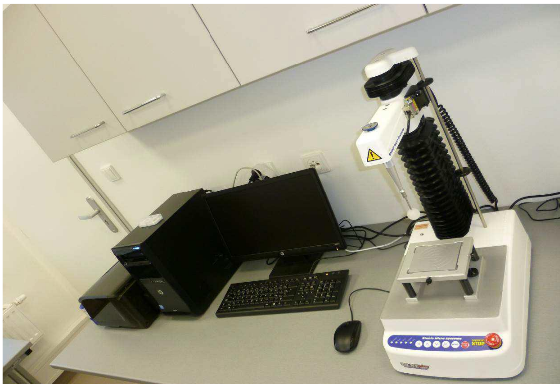
Obr. 2 Texturometr TA.XTPlus (Stable Micro Systems, Godalming, England) s kulovou sondou (Foto autor).
