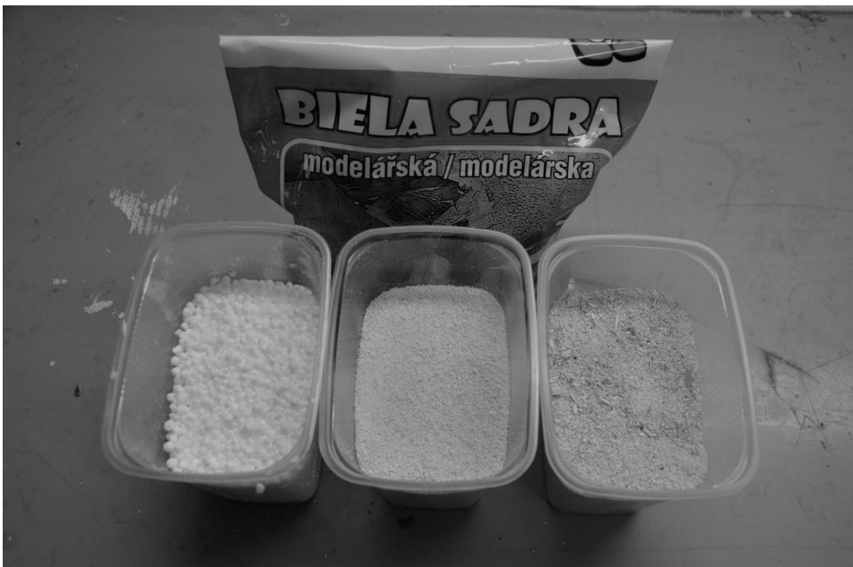
Fig. 11. Filling mixture made of plaster and sawdust can be lightened up with pearlite or polystyrene.
