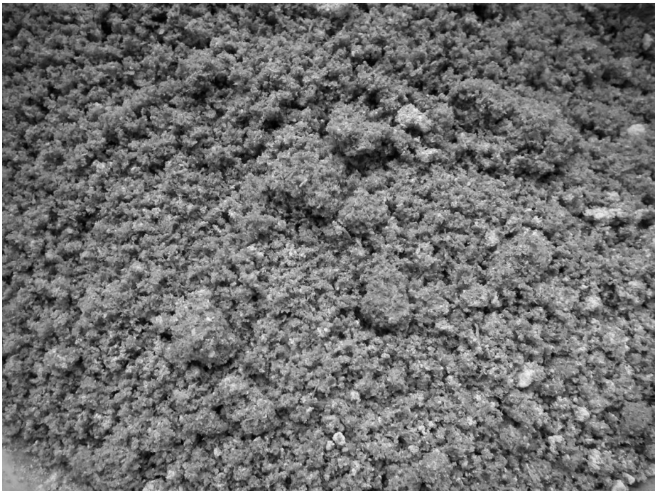
Fig. 15. Finished loose filling mixture made of fine sawdust and plaster.
