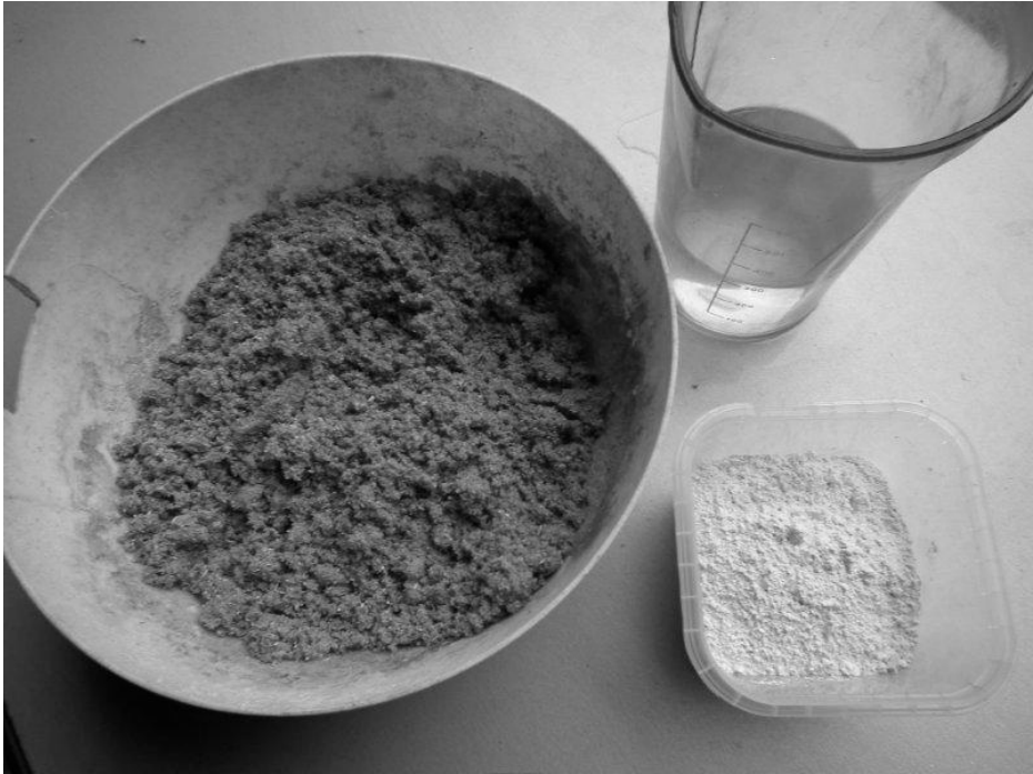
Fig. 14. Sawdust remains loose even after moistening.
