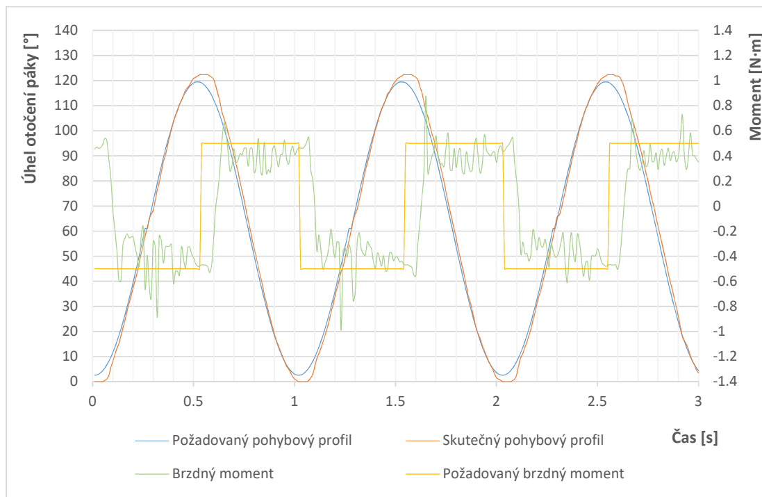
Obr. 55 Servomotor (GPA 3.1, Mode 3 – 0,5 N·m, Switch polarity)
