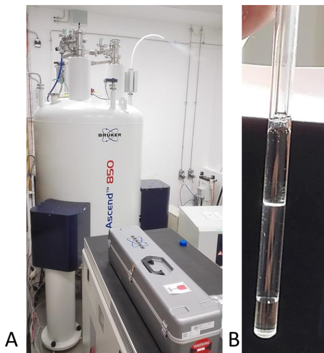
Figure 12. A. Institute of Organic Chemistry and Biochemistry of the CAS, Prague. Magnet: Bruker superconducting 850 MHz, Ascend™, console: Avance III HD 850. B. The sample of DmxA enzyme in the glass tube. Pictures prepared by K. Doleželova.
