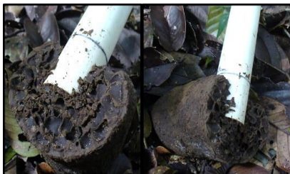
Figure 6. Reference soil core taken from Dicuspiditermes minutus mound to obtain specific volumetric weight for estimation of total mound weight.
