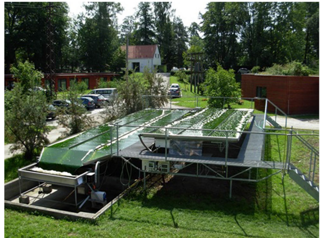
Fig. 10 Outdoor thin-layer cascade for cultivation of microalgae constructed from stainless steel. It has an area of 90 m 2 and can be operated with a volume between 500 and 1500 L. The surface-to-total-volume ratio can be operated in the range between 60 and 180 1/m corresponding to a layer thickness of suspension between 5 and 15 mm
