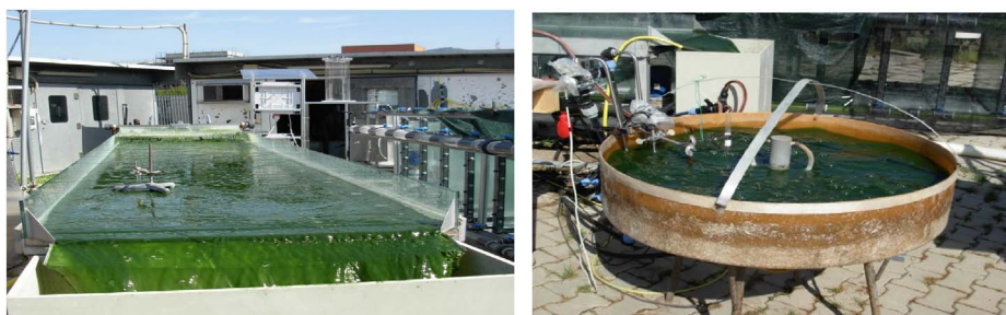
Fig. 1. Cultivation units used in trials – inclined thin-layer cascade (TLC; left) and open circular pond (OCP; right).
