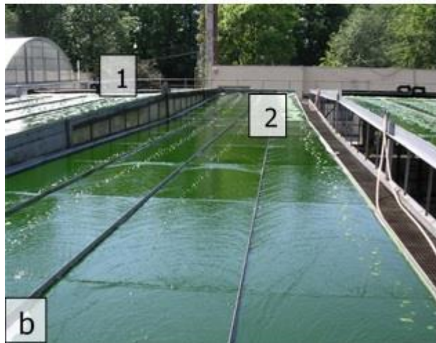
Fig. 14 The third generation of outdoor cascades with about 660 m 2 . It consists of three units (a) with each 220 m 2 arranged as a cascade of four planes arranged symmetrically in a roof-shape design (b).
