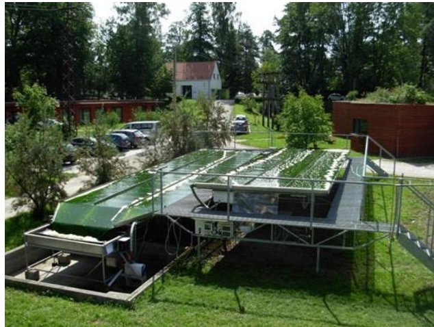
Fig. 15 The latest generation of cultivation unit with the area of 90 \text{ m}^2 can be operated with a volume between 500-1500 L. The total surface to volume ratio can be operated in the range between 60 and 180 \text{ m}^{-1} .
