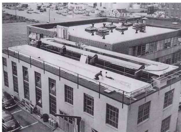
Fig. 1 One of the first pilot-scale units (about 4000 L) was devised and tested at Arthur D. Little, Inc. in Cambridge, Massachusetts in collaboration with the Carnegie Institution in 1951. The photobioreactor was formed by a loop of thin-walled polyethylene tube of a 7–8-cm depth with continuous circulation of the culture by a pump
