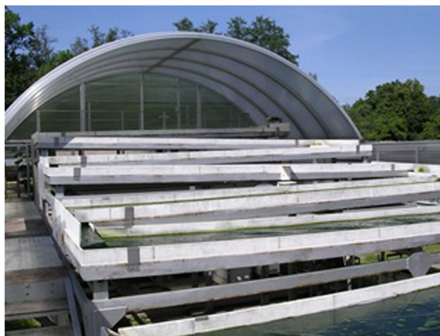
Fig. 11 A multiple-lane cascade system constructed as a semi-closed system placed in a greenhouse (Institute of Microbiology, Třeboň, Czech Republic). The culture was circulated over the cascade of 8 smooth polypropylene platforms arranged in a meandering way with a declination of 1.6% (total area of 56 m 2 and total volume of 500–600 L) which were connected by troughs. The flow velocity was about 0.5 m/s with a culture layer thickness of about 6–7 mm
