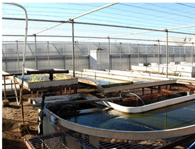
Fig. 12 Labyrinth-like thin-layer system of 32 m 2 in area with total volume of 1200 L was constructed at the University of Almería, Spain (Morales-Amaral del Mar et al. 2015). The layer thickness of culture is about 20 mm. The culture is pumped from the aerated tank to the first layer using a low-stress centrifugal pump; then it is circulated by gravity at 0.2 m/s until it returns back to the tank
