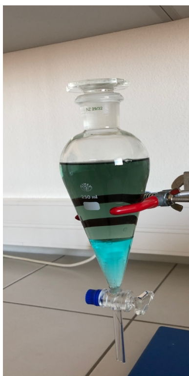
Fig. 4.1.: Typical result of the chloroform extraction
