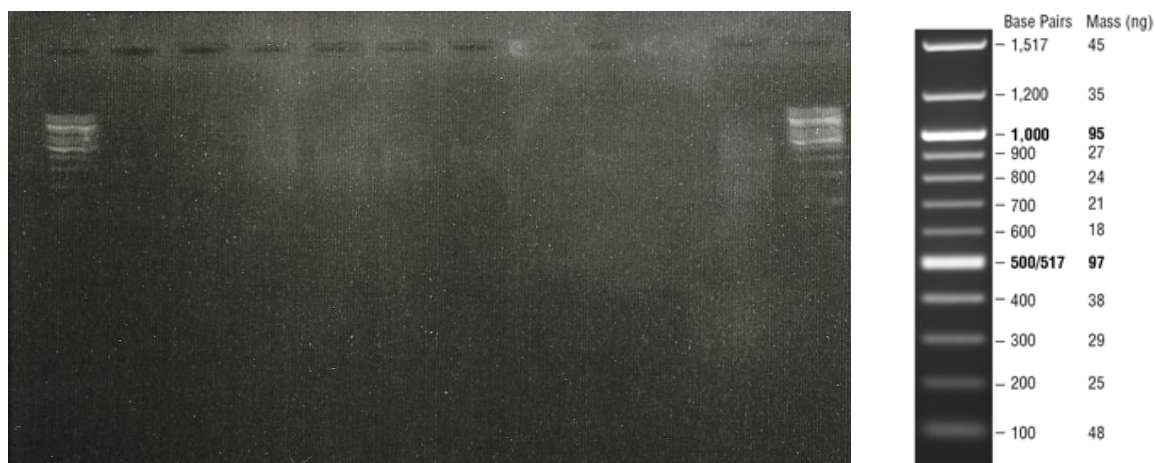
Fig. 5. The first 1.5 % TAE agarose gel of the third attempt. Only every second well was filled with samples. On the right is the 100 bp DNA Ladder, observed through ethidium bromide staining on a 1.3 % TAE agarose gel, with mass values assigned to each lane (0.5 \mu g per lane). The last and first wells were filled with GeneRule 1 kb DNA Ladder by Thermo Scientific. The gel was subjected to UV light at 268 nm for 5 minutes. The base pairs were visualized by 6x DNA Nucleic Acid Stain in 10 000 x in DMSO. As can be seen, by the ladders, the gel electrophoresis was terminated too early before the samples could separate enough.
